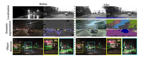
**Fig. 1.** Our ForkGAN can boost performance for multiple vision tasks with night to day image translation: localization (by SIFT point matching between daytime and nighttime images), semantic segmentation and object detection (by data augmentation) in autonomous driving (results are all shown on the nighttime images).
