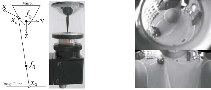
Fig. 1. Left: Diagram and physical catadioptric camera system. Upper right: catadioptric image captured from the camera, lower right: transformed image using a virtual cylindrical camera.
