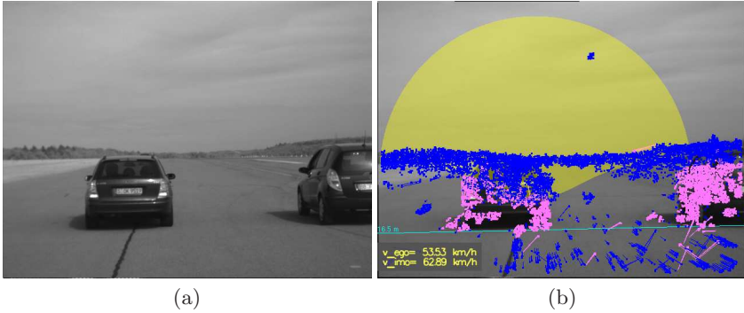
Fig. 9. Experimental result. (a) Original image with two moving vehicles in front. (b) The semi-transparent yellow region shows the image region where the motion is not detectable. The measured optical flow vectors are classified as static (blue / dark) and moving (magenta / bright).
