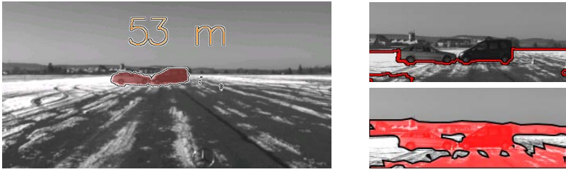
Fig. 4. Motion segmentation and distance estimation for different color obstacles in 53 m distance from monocular vision alone. The camera translation was 2.6 m between the frames. The right plots show the region of interest with motion segmentation ( top ) and gray value segmentation ( bottom ) for the same frames. Clearly, gray value segmentation is not suitable for the segmentation of different colored obstacles in scenes with arbitrary background.
