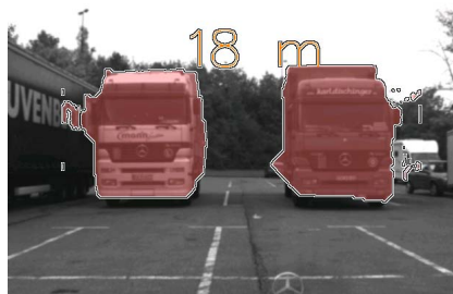
Fig. 6. Detection of a gap between obstacles. Taking the center of mass for the distance measurements results in one detected object. The gap between the two trucks is ignored.
