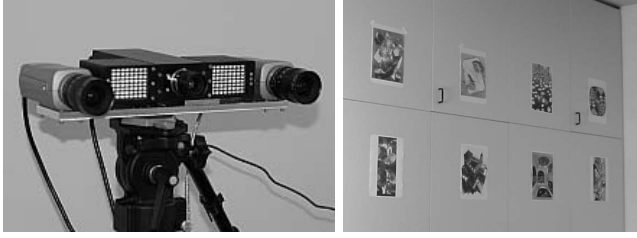
Fig. 3. Left: The Rig used to obtain the results. It consists of two color cameras that frame the PMD-Camera. Right: One of the stereo images.
