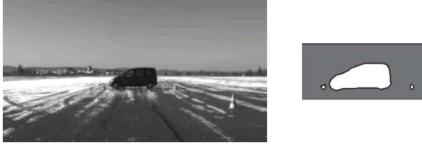
Fig. 1. Motion segmentation of a stationary obstacle in 36 m distance from monocular video. Notice the two cones, which are difficult to capture by means of their gray value.
