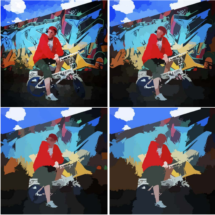
Fig. 1. Sample quick shift results. Increasing \sigma smooths the underlying estimate of the density, providing fewer modes. Increasing \tau increases the average size of a region as well as the error in the distance estimate. The top row of images have \sigma = 2 , the bottom row \sigma = 10 . The left column has \tau = 10 and the right \tau = 20 .
