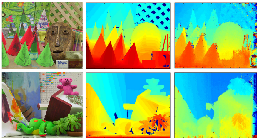
Fig. 6. Results of SGM GPU implementation using the Middlebury Stereo Datasets: the left images are related input images, the middle images are the ground truth depths and the right images are the GPU results
