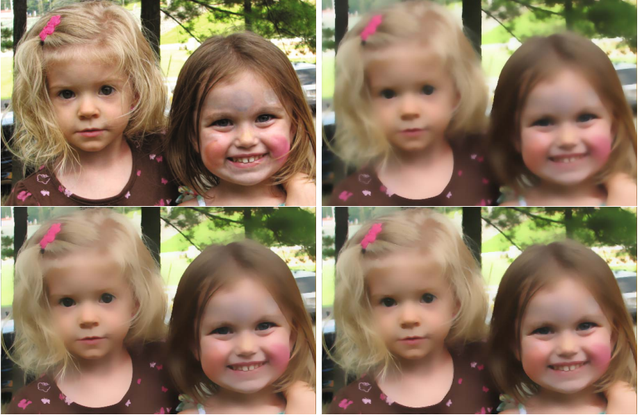
Fig. 7. Top: left: original image, right: RGB bilateral filter. Bottom: left: CIELAB bilateral filter, w = 11 , \sigma_d = 5 , \sigma_r = 0.1 , right: our method, \epsilon = 0.1 .
