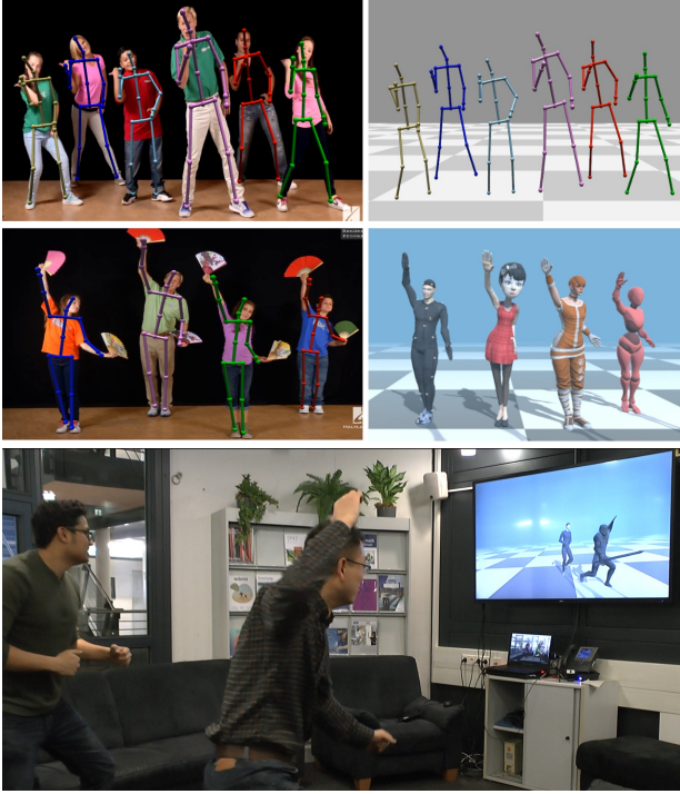
Fig. 7. Live Interaction and Virtual Character Control: The temporally smooth joint angle predictions from Stage III can be readily employed for driving virtual characters in real-time. The top two rows show our system driving virtual skeletons and characters with the motion captured in real time. On the bottom, our system is set up as a Kinect-like game controller, allowing subjects to interact with their virtual avatars live. Some images courtesy Music Express Magazine [2013a; 2013b]. See the accompanying video and the supplemental document for further character control examples.
