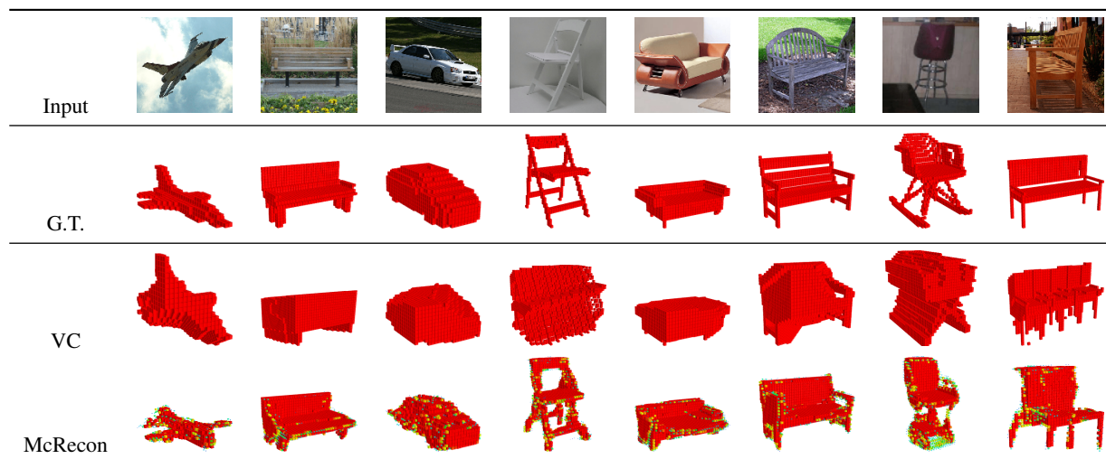
Figure S3. Qualitative results of real image reconstructions on ObjectNet3D. The results hints that our network successfully carved out concavity, which cannot be learned from mask supervision. Please note that voxel carving requires camera parameter at test time while ours does not.
