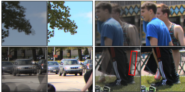
Figure 7: Small displacements in the acrobat and street traffic scenes. The left of each pair is the mean registered input image, thus ghosting shows small displacements. Our method on the right of each pair handles shifts of just a few pixels between exposures.
