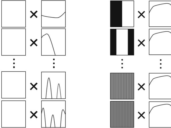
**Fig. 3.** Projected images: (left) nine basis images for spectral reflectance estimation (nine spectral basis light sources with a white image), and (right) eight stripe images for 3D shape reconstruction (eight stripe pattern images with a white light source).
