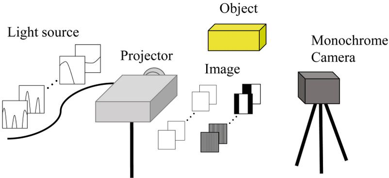
**Fig. 2.** Overview of our measurement system
