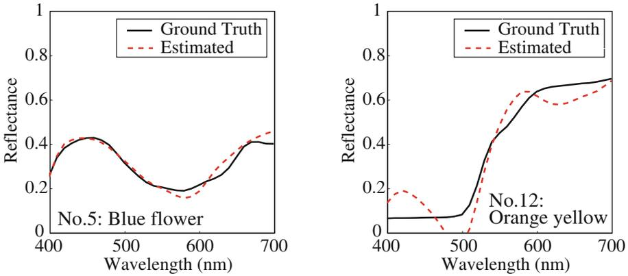
**Fig. 6.** Estimated spectral reflectances: (left) reflectance of ColorChecker No.5 which is estimated with the minimum color difference ( $RMSE = 0.024$ ,  $GFC = 0.9978$ ,  $\Delta E_{ab}^* = 1.25$ ), and (right) reflectance of ColorChecker No.12 which is estimated with the maximum color difference ( $RMSE = 0.074$ ,  $GFC = 0.9872$ ,  $\Delta E_{ab}^* = 10.96$ ).
