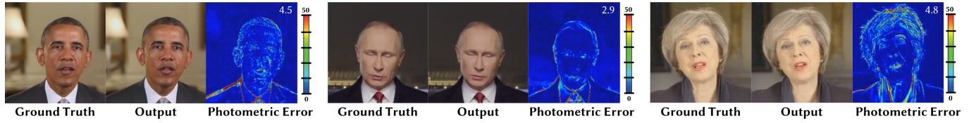
Fig. 7. Quantitative evaluation of the photometric re-rendering error. We evaluate our approach quantitatively in a self-reenactment setting, where the ground-truth video portrait is known. We train our rendering-to-video translation network on two thirds of the video sequence, and test on the remaining third. The error maps show per-pixel Euclidean distance in RGB (color channels in [0, 255] ); the mean photometric error of the test set is shown in the top-right. The error is consistently low in regions with conditioning input, with higher errors in regions without conditioning, such as the upper body. Obama video courtesy of the White House (public domain). Putin video courtesy of the Kremlin (CC BY). May video courtesy of the UK government (Open Government Licence).
