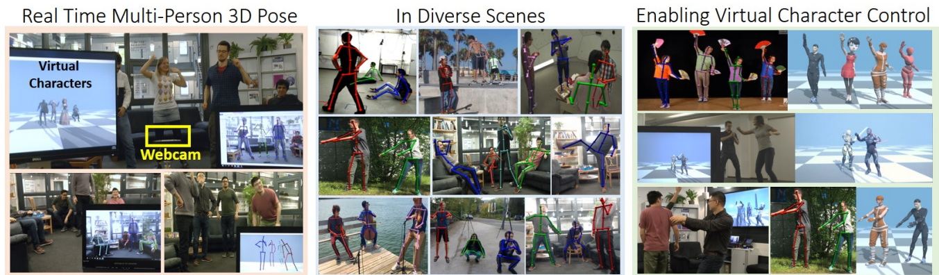
Fig. 1. Our real-time monocular RGB based 3D motion capture provides temporally coherent estimates of the full 3D pose of multiple people in the scene, handling occlusions and interactions in general scene settings, and localizing subjects relative to the camera. Our design allows the system to handle large groups of people in the scene with the run-time only minimally affected by the number of people in the scene. Our method yields full skeletal pose in terms of joint angles, which can readily be employed for live character animation. Some images courtesy [KNG Music 2019], [Music Express Magazine 2013a]. 3D characters from Mixamo [Adobe 2020].
