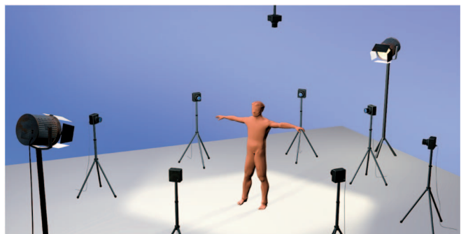
Fig. 3. Illustration of camera and light source arrangement.
