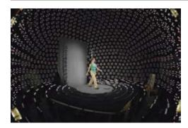
The lighting apparatus, treadmill, and turntable used for capturing human locomotion from multiple viewpoints under time-multiplexed lighting.
