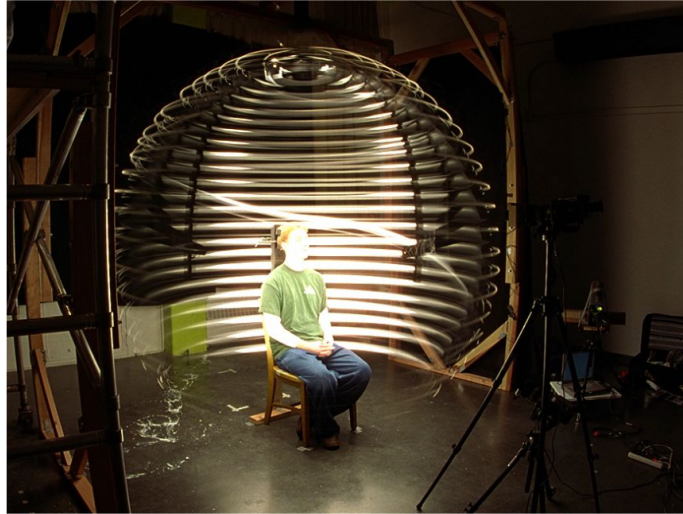
This 1-minute exposure shows how Light Stage 1 moved a small spotlight around a person's head during the capture process. Image courtesy Paul Debevec.
